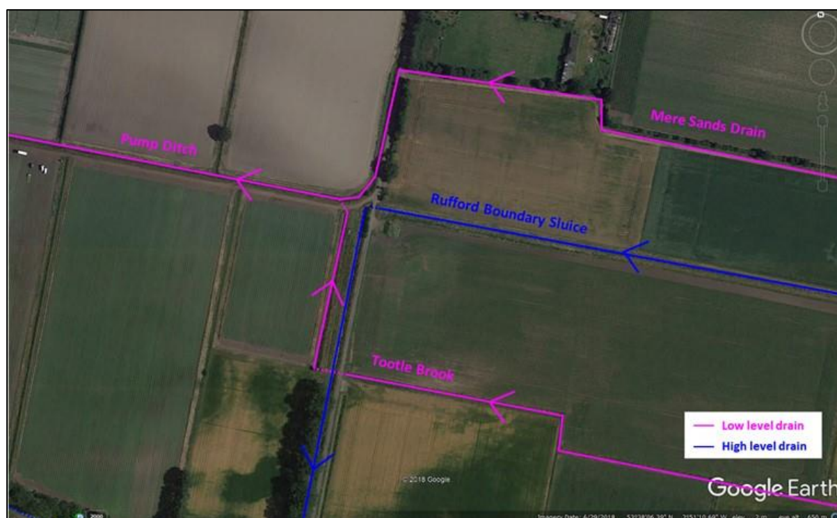
Figure 3-7 Drainage network at Sandy Way
